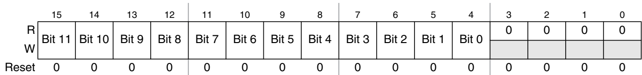
Figure 13-14. Left justified ATD conversion result register (ATDDR n )
