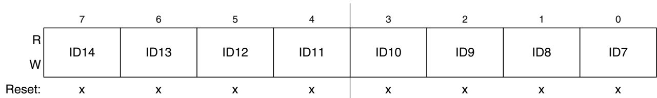
Figure 16-28. Identifier Register 2 (IDR2) — Extended Identifier Mapping
