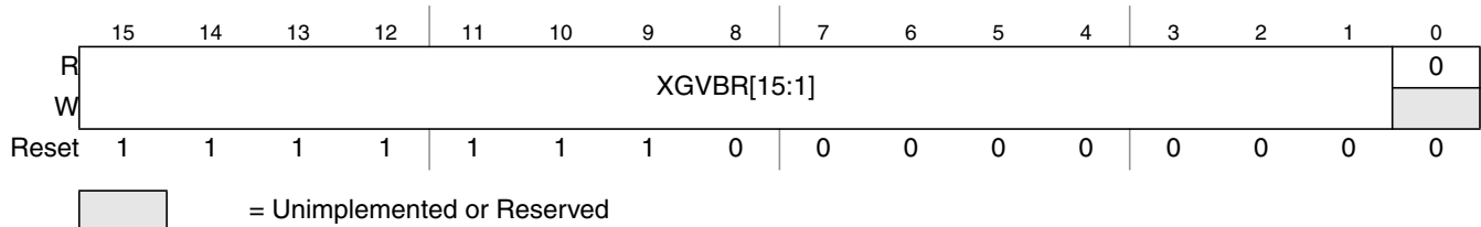
Figure 10-9. XGATE Vector Base Address Register (XGVBR)
